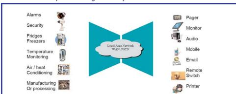
Alarms can originate from a range of inputs such as security, air-conditioning, manufacturing or processing, and are received at a central location. Alarm messages are sent via the local area network out to an alarm message recipient, such as a Pager, PC, Mobile, Printer, Display Panel, or PMR Handset. Messages may be text, audio, visual or a combination.
