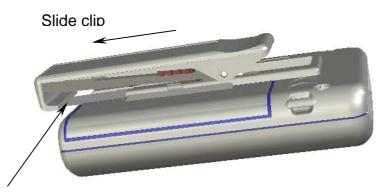
Metal back-plate (insert blade under this edge)
