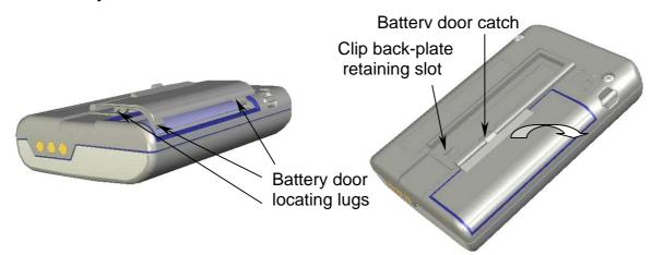
Ensure that the battery door lugs are lifted clear of the case and remove the door. Remove the battery by placing your forefinger onto the positive end-cap and lifting the battery upwards, at the same time pushing slightly backwards against the negative contact spring. Battery replacement is the reverse sequence. Observing the correct polarity, place the battery against the negative contact spring and compress slightly, at the same time pushing the
